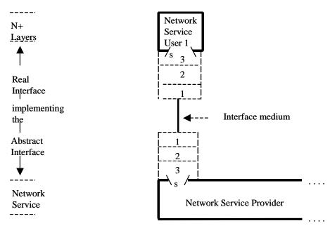
**Figure 3**: Network Service User connected to the Network Service Provider by a real interface which is built up of three layers of interface protocol and uses a physical medium.
