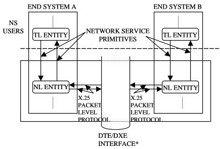
\* this interface consists of 0 or more network layer entities providing a network layer relay function
