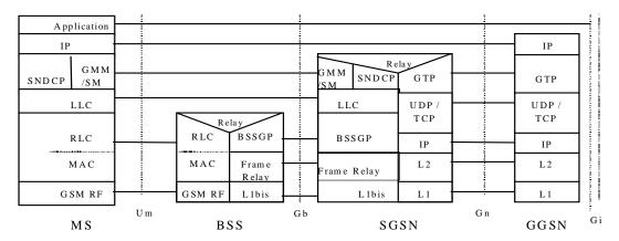
FIGURE 3. GPRS Transmission/Signalling Planes From MS to GGSN
