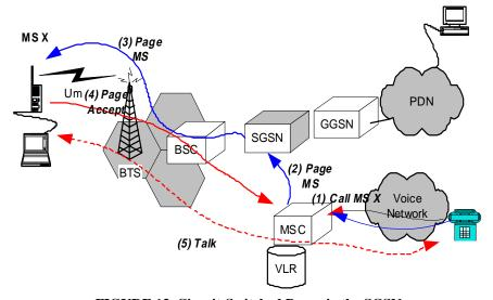
FIGURE 13. Circuit-Switched Page via the SGSN
