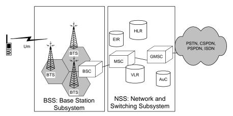
**FIGURE 1. GSM Network Architecture**
