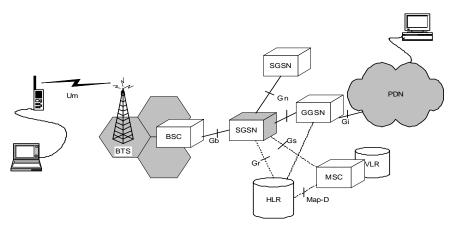
FIGURE 2. Logical architecture of GPRS Network
