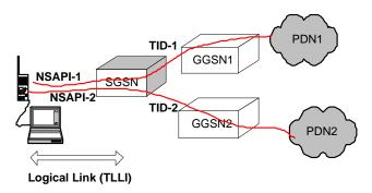
FIGURE 10. A MS with two PDP Contexts Active
