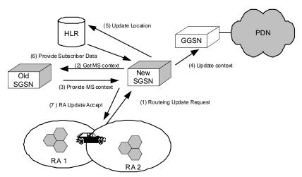
FIGURE 9. Inter-SGSN Routeing Update Procedure (simplified)
