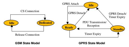
FIGURE 7. GSM and GPRS Functional State Models
