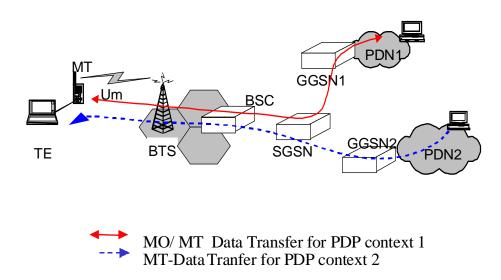
FIGURE 11. End-to-End Packet Switching for a MS in the Home Network
